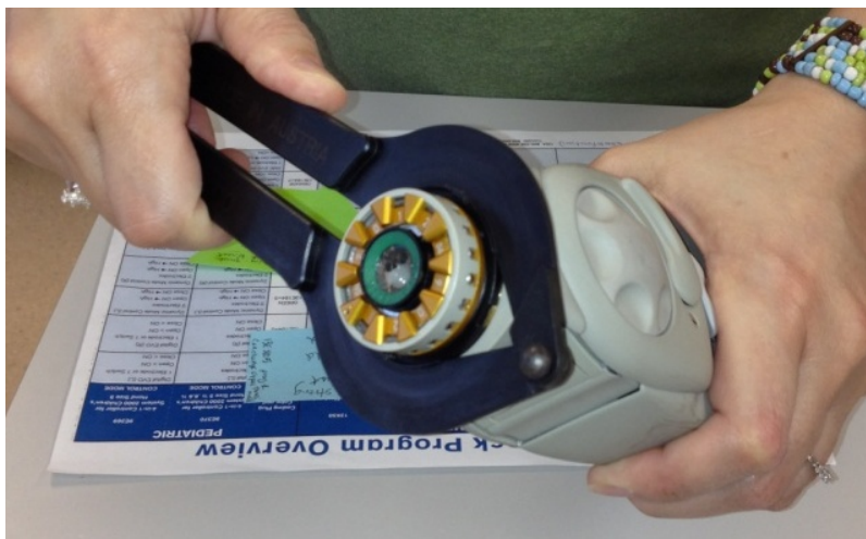
Fig. 3 This shows the newer version (706Z10) Pincer to be used with the black plastic friction ring (1.3) of the Greifer.
