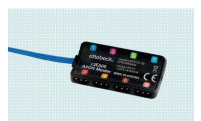
The AxonMaster as the central control unit of the Axon-Bus system is connected directly to the AxonEnergy Integral. It receives and processes control signals from the user and transmits them to the respective prosthesis components. This allows the user to control the hand movements and switch between the prosthesis components directly and reliably. The AxonMaster stores all control parameters of the prosthesis system.
