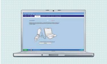
In order to establish individual user settings for the prosthesis components, the myo-signal must be evaluated. This is done using the AxonSoft adjustment software, which is integrated into the Ottobock Data Station.
