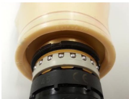
Figure 1 – Bearings are engaged
