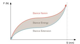
The kinetic energy the amputee applies to the EBS unit in stance flexion (red line) is not fully returned in the subsequent stance extension movement (blue line).
