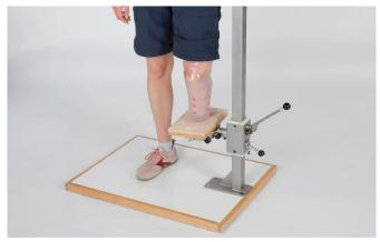
Check the fit of the prosthetic socket as described in the following steps. Correct any deviations.
