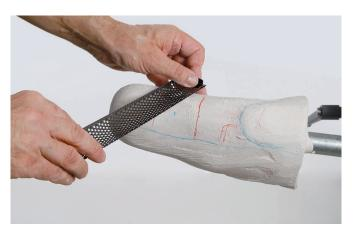
Reduce the distal end of the model by **5 mm** to **8 mm** without changing the shape.
