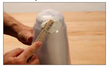
Isolate the vacuum formed socket in the area of the distal base with 627B40 PE Adhesive Tape. Fill all undercuts in the distal base and metal dummy areas with light putty. This serves for easy removal of the flexible inner socket from carbon frame.
