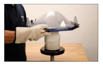
Vacuum form the test socket with Thermolyn rigid 616T52=\* or clear 616T83=\* in usual way.
