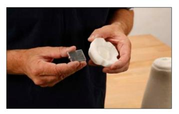
Slide metal dummy into the recess on distal base.
