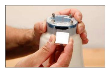
Carefully isolate metal dummy with silicone grease and slide the dummy into the recess. Remove the screw. Carefully isolate the thread with silicone grease and protect against resin penetration with 636K8=\* Plastaband.
