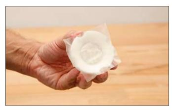
Isolate the concave side with 616F8 Coroplast PVC Adhesive Tape.
