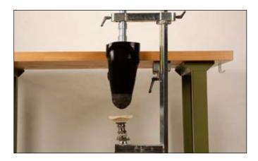
Laminate the socket according to the patient's weight and functional requirements. Attach the socket adapter to the socket clamped in the transfer apparatus. Sand and laminate the socket adapter in usual way.
