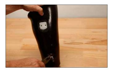
Cut out as necessary after the lamination resin has hardened. Cut open the recess area on the distal base where the metal dummy is embedded, remove Plastaband, screw in the M4 screw and pull the metal dummy out of the distal base. You can facilitate pulling out the dummy by lightly heating the laminate. Grind away the 4R162 Dummy and remove the Philips screws. Dismantle the 4R161 Lamination Kit. Remove the socket from plaster model.
