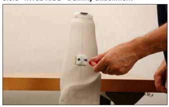
Determine the position of the proximal socket opening along the line marked according to section 5.3.2 which points in direction of the strap outlet. It should be located at a maximum of 2.5 cm (1") distally from ischial tuberosity. This opening may never be positioned higher than the lowest point of the liner brim. Screw the 4R162 Dummy on the model on the previously marked position. Make sure that the recessing in the dummy corresponds to the previously marked line.
