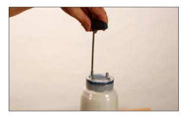
Carefully isolate all screws with silicone grease. Screw the spacer screws fully into the distal base.
