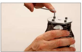
Isolate the lamination disk included in the 4R161 Lamination Kit with silicone spray or silicone grease and fix the disk on spacer screws using screws already covered with silicone grease. Cover the hex socket with 638K8=\* Plastaband to prevent from resin penetration. Pull over another PVA bag. Laminate in usual way.
