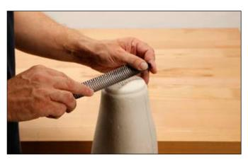
Slightly roughen the plaster model surface around the 6 mm ( $^{1}/_{4}$ ") dia. hole.
