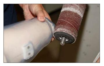
After cooling down cut open the socket on the proximal marked socket brim. Grind away the metal dummy inserted into the recess and the convexness caused by the 4R162 Dummy.
