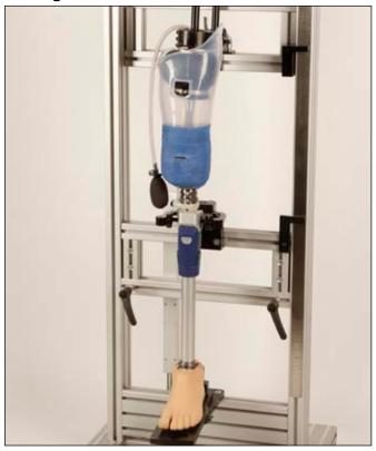
Bench alignment of the prosthesis PROS.A.Assembly 743A200. The prosthesis is assembled for example with the 5R1=6 Attachment Block, 3R90 Knee Joint with Friction Brake and 1D35 Dynamic Motion.
