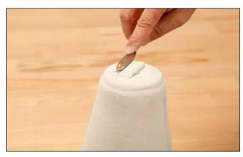
Apply a bit of mixed plaster into the hole and around the hole onto the roughened area of the plaster positive.
