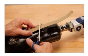
Cut the strap 1 cm proximally of the distal recessing. Melt together the cutting edge with a cigarette lighter and reinforce the edge with a seam if necessary.
