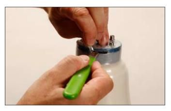
Cut away the 627B40 PE Adhesive Tape in the recess area.
