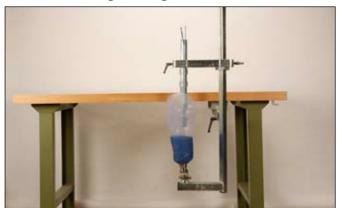
Once the dynamic trial fitting has been completed, separate the prosthesis directly above the knee joint and clamp the prosthesis into the 743A160 Transfer Apparatus.
