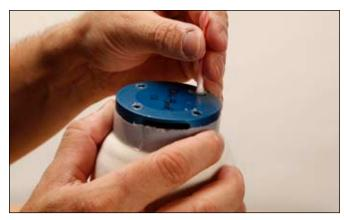
Isolate all holes on distal base with 633F11 Silicone Grease.
