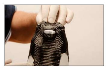
Cut the spacer screws and metal dummy open in every step.
