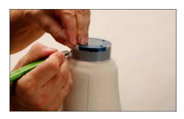
Cut the nylon stockinette circularly at the proximal edge of the recess.
