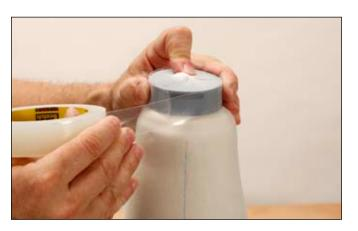
Cover the nylon stockinette on distal base with 627B40 PE Adhesive Tape up to the recess.
