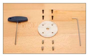
Dismantle the 4R161 KISS® Lamination Kit . Use Allen wrench, size 3 mm for loosening the black screws and Allen wrench, size 4 mm for spacer screws.
