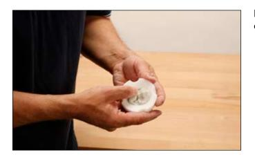
Fill the space along the rounded surface on the concave side of the distal base with 636K6 Plasticine.
