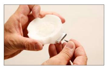
Fill the thread with 636K8 Plastaband.
