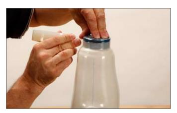
Pull over PVA bag and turn on vacuum pump. Wrap 627B40 PE Adhesive Tape around the distal base so the latter can be easily replaced if need be later on. Cut away the excessive PVA bag and wrap around another layer of the PE adhesive tape.
