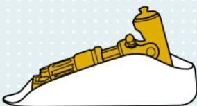
**EN** Unscrew the foot pads and screw the footshell to the foot. Secure the supplied screws with Loctite in addition. Now the user can put on the snowboarding boots directly.
